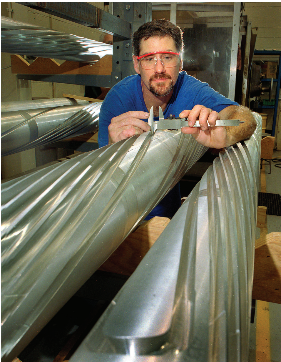
FIGURE 5.4 Aluminum tubes with spiraling grooves were used for the construction of 48 full-twist superconducting helical dipoles for the Siberian snakes and spin rotators that allowed the acceleration and collision of up to 250 GeV polarized protons at the Relativistic Heavy Ion Collider at Brookhaven National Laboratory. SOURCE: Brookhaven National Laboratory.
