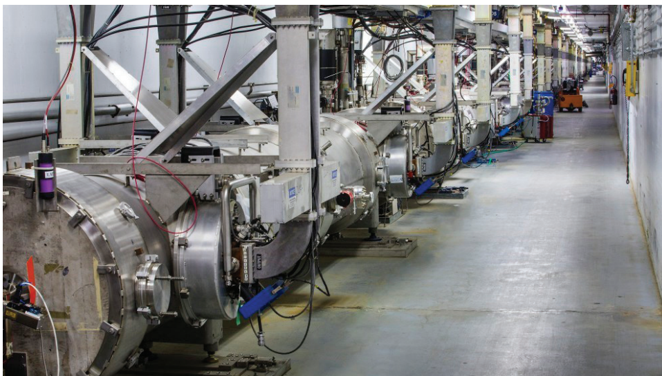
FIGURE 5.2 A view of the Continuous Electron Beam Accelerator Facility accelerating structures, recently upgraded to provide 12 GeV beams. SOURCE: Thomas Jefferson National Accelerator Facility, https://www.jlab.org/ , accessed August 13, 2018.
