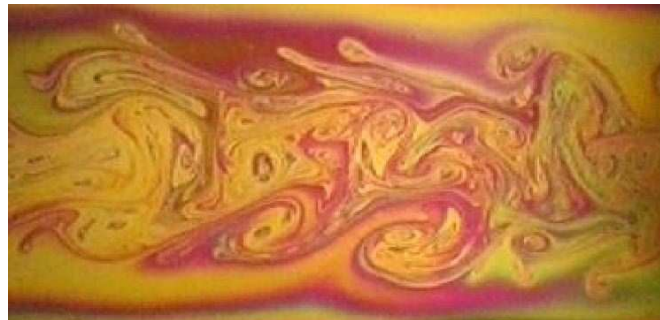
FIG. 1: Turbulence in a soap film behind a one-dimensional vertical grid (courtesy Hamid Kellay, Université de Bordeaux I, France).
